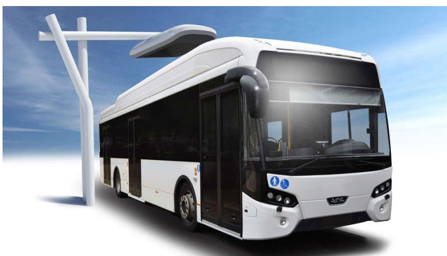
Electric Bus using a Pantograph Fast Opportunity Charger
