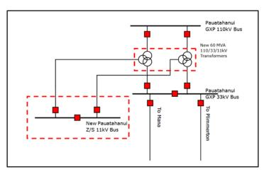
Figure C-14 Pauatahanui Zone Substation Sub transmission Supply
