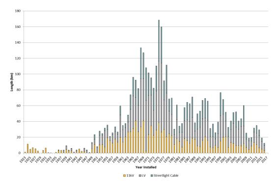
Figure 6-45 Age Profile of Distribution Cables
