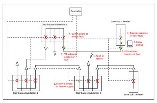
Figure C-9 Distribution Level Remote Switching Architecture
