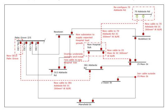
Figure C-5 Proposed Palm Grove Zone 1 Ring Reinforcement
