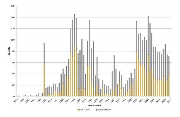
Figure 6-47 Age Profile of Distribution Transformers
