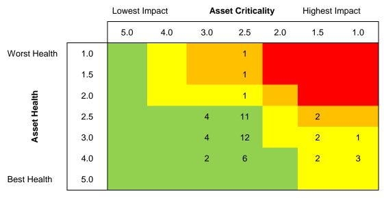
Figure 6-18 Power Transformer Health-Criticality Matrix
