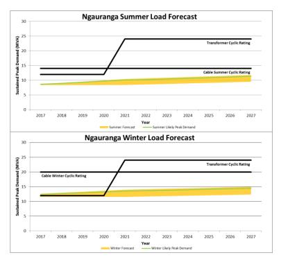
Figure C-18 Ngauranga Load Forecast following transformer replacement
