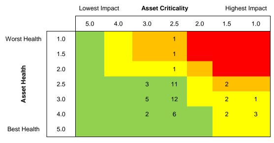
Figure 6-2 Health-Criticality Matrix (Power Transformers example)
