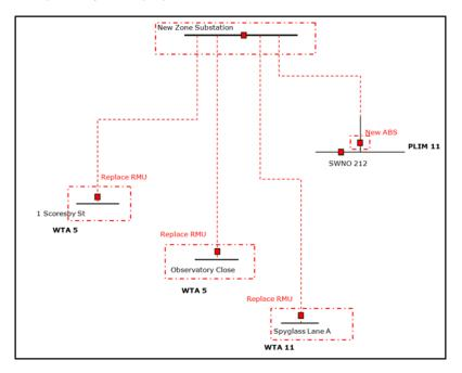
Figure C-12 Proposed Distribution Inter-connectivity
