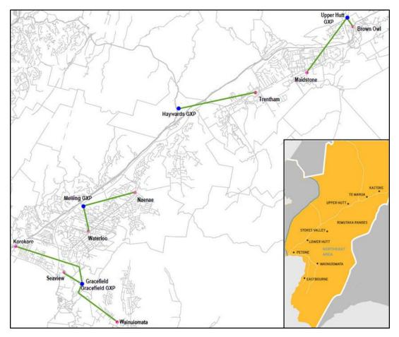
Figure 3-10 Wellington Northeastern Area Sub transmission Network
