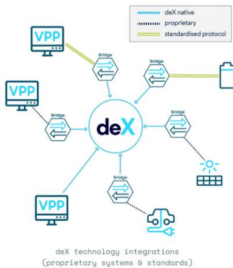
Figure 3: deX API and 'bridging' communications schematic
